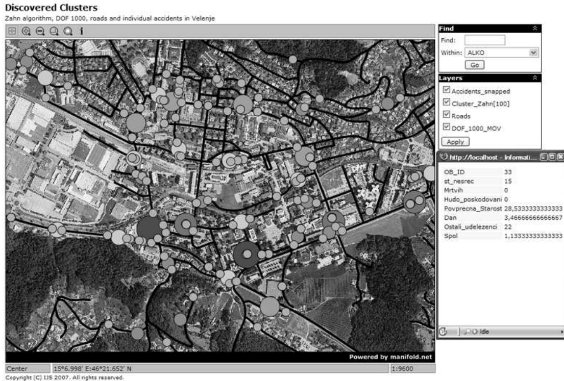
Figure 15: Discovered clusters with the Zahn algorithm and individual accidents snapped onto roads, visualized with the Internet Map Server (Digital OrtoFoto as an underlayer).
